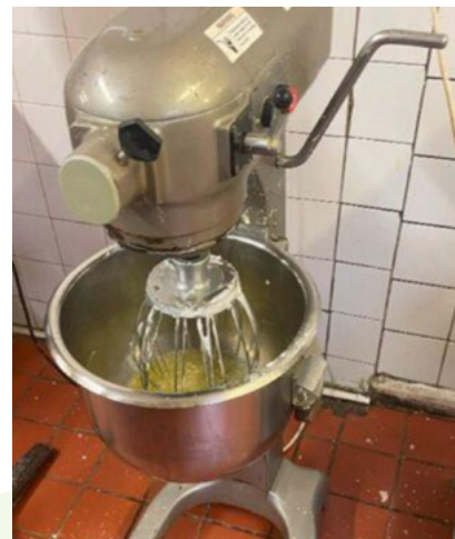
Food mixer missing a guard
